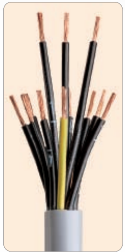
Flexible Stranded Bare Copper Conductors, PVC Insulated Grey PVC Outer Sheath, Black numbered Cores with Green/Yellow Earth Core VDE 0250/0281
